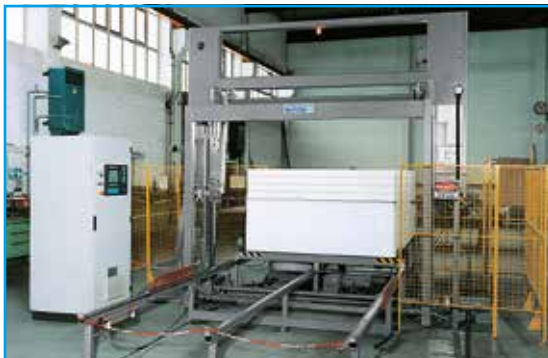
W 21 automatic horizontal splitting and stacking machine with sliding table.
