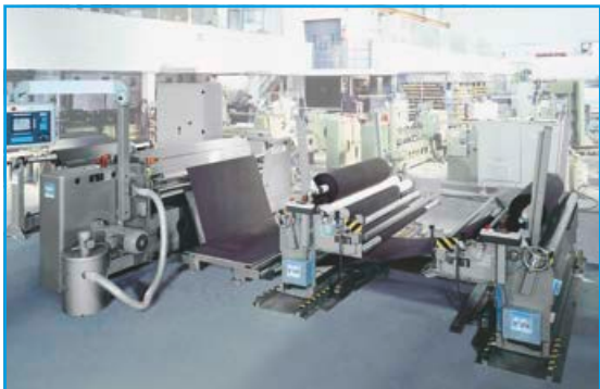
Splitting Machine G 11 with wind-up and wind-off device.
