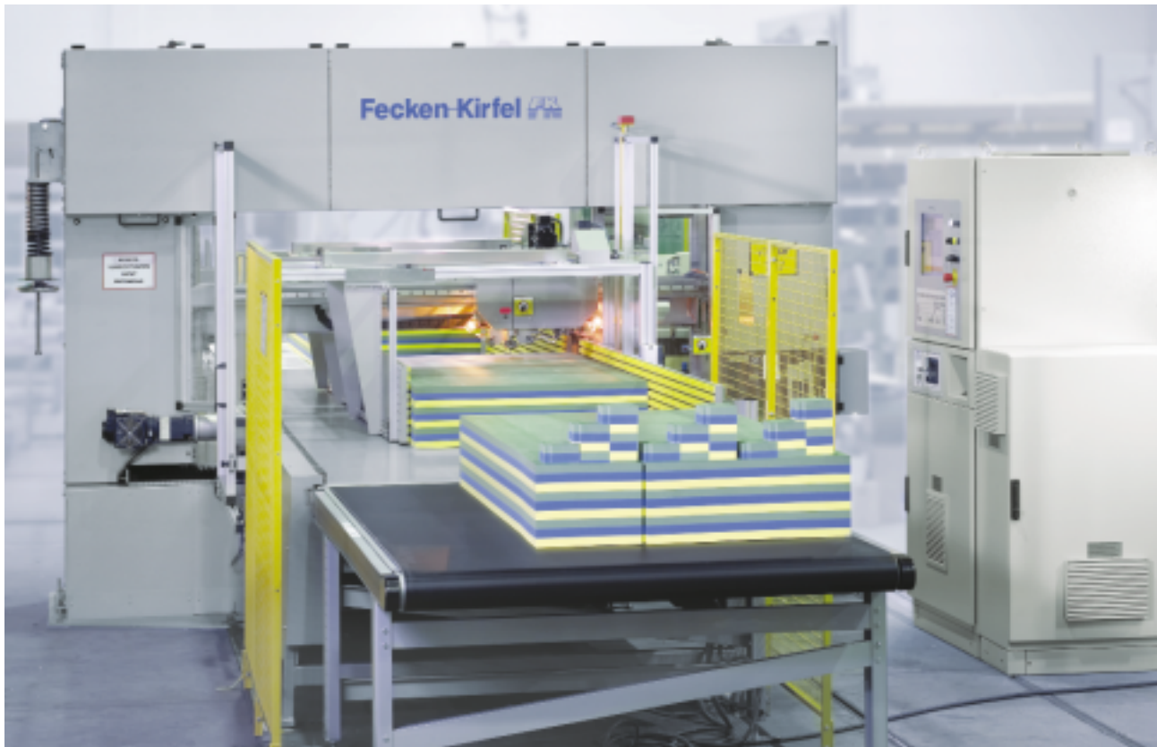
F 62 with automatic loading and unloading device
